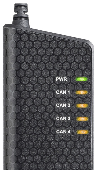
Figure 4: LEDs on the Kvaser USBcan Pro 4xCAN Silent.
