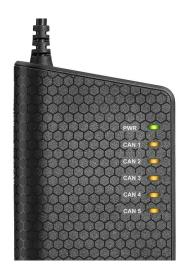
Figure 4: LEDs on the Kvaser USBcan Pro 5xCAN.
