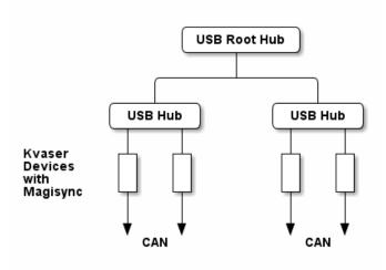
Figure 8: An example setup where all devices are synchronized via MagiSync.
