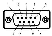
Figure 6: The male D-SUB 9 connector pin numbers
