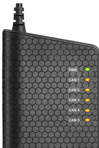
Figure 4: LEDs on the Kvaser USBcan Pro 5xCAN.
