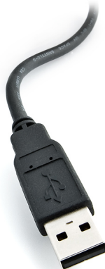
Figure 2: A standard USB type "A" connector.
